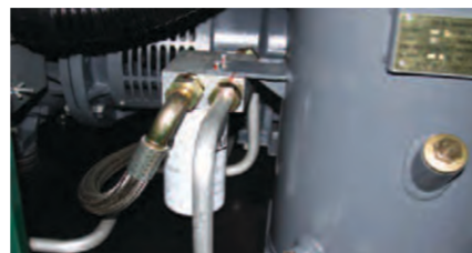
Lubricant filter assembly features a spin-on,
