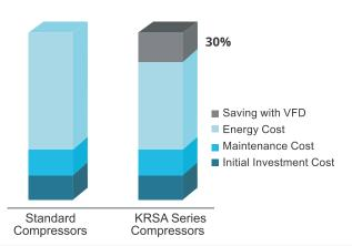
KRSA series up to 250kW are also available with Permanent Magnet Variable frequency (PMV) drive option for best in class part load efficiency,
